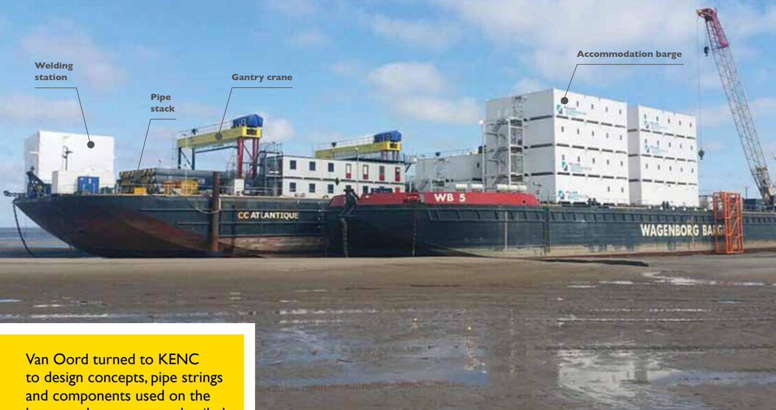
Van Oord turned to KENC to design concepts, pipe strings and components used on the barge, and to carry out detailed engineering and structural analysis of the barge.
